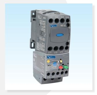
E&A introduces REO range of Electronic Overload Relays to complement the MO range of contactors. REO electronic overload relays are available in 2 version and in 2 frame size. REO range of Electronic Overload Relays provide protections against overload, single phasing, locked rotor and ground fault and are modular in design.
